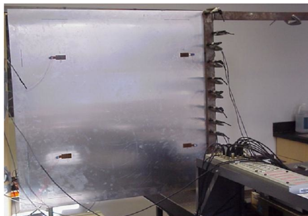
Figure 3: Vibrations in a plate occur due to various disturbances. In this apparatus the vibrations are controlled via the piezo-electric patches shown. (Photo by courtesy of Prof. M. Demetriou, Worcester Polytechnic University.)
