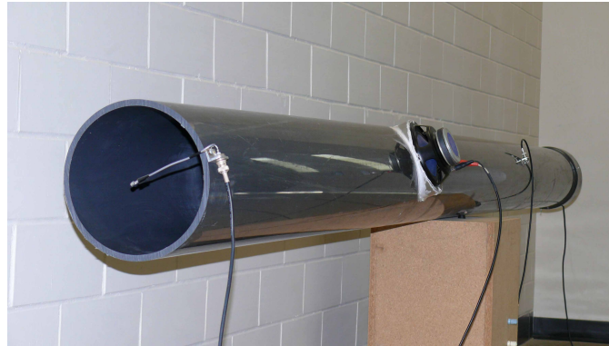
Figure 2: Acoustic noise in a duct. A noise signal is produced by a loudspeaker placed at one end of the duct. In this photo a loudspeaker is mounted midway down the duct where it is used to control the noise signal. The pressure at the open end is measured by means of a microphone as shown in the photo. (Photo by courtesy of Prof. S. Lipshitz, University of Waterloo.)
