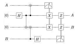
In the above, circuit convention follows Nielsen and Chuang. In particular, a vertical double line connecting a measurement box (in the computational basis) to a unitary U means that "conditioned on the measurement outcome being 1, perform U, otherwise do nothing". X, Z, H are the Pauli-x, Pauli-x, and the Hadamard gates.
