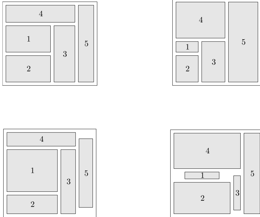
Figure 8.20 Four instances of an optimal floor plan, using the relative positioning constraints shown in figure 8.19. In each case the objective is to minimize the perimeter, and the same minimum spacing constraint between cells is imposed. We also require the aspect ratios to lie between 1/5 and 5 . The four cases differ in the minimum areas required for each cell. The sum of the minimum areas is the same for each case.
