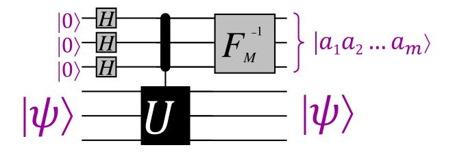
If  $\phi = 0. a_1 a_2 \cdots a_m$  then the above procedure yields  $|a_1 a_2 \dots a_m\rangle$  (from which  $\phi$  can be deduced exactly)
