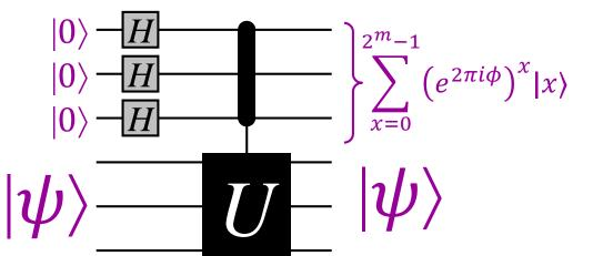
$\mapsto (|0\rangle + e^{2\pi i\phi}|1\rangle + (e^{2\pi i\phi})^2|2\rangle + (e^{2\pi i\phi})^3|3\rangle + \dots + (e^{2\pi i\phi})^{2^{m-1}}|2^m-1\rangle)|\psi\rangle$
