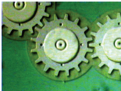
Fig. 15. Gears, showing mechanical play ( http://www.sfu.ca/adm/gear.html , used by permission, Robert Johnstone, SFU). Since the gears are not perfectly meshed, when one gear turns there is a period of time when the driven gear is stationary before it engages and is turned by the first gear.
